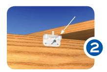
Step 2: Using the Invisi-Fast<sup>TM</sup> Angle with spacer, slide the convenient overhang tabs under your first deck board for hands free attachment. Then using an approved deck screw, fasten the Invisi-Fast<sup>TM</sup> Angle to the joist using a lower hole.
