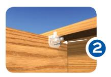
Step 2: Using the Invisi-Fast<sup>™</sup> with spacer, slide the convenient Overhang Tabs under your first deck board for hands free attachment. Then, using an approved deck screw, fasten the Invisi-Fast<sup>™</sup> to the joist using a lower hole.
